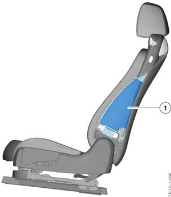
F12 Seat with side head airbag
